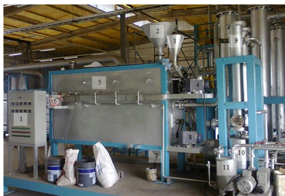
Fig. 1: Schematic diagram of experimental setup: 1) control panel and switchboard 2) biomass hopper 3) catalysts hopper 4) motor screw I 5) pyrolysis reactor 6) burner 7) charcoal outlet slit 8) motor screw II 9) condenser 10) bio-oil stock 11) gases storage and recovering in the system.
